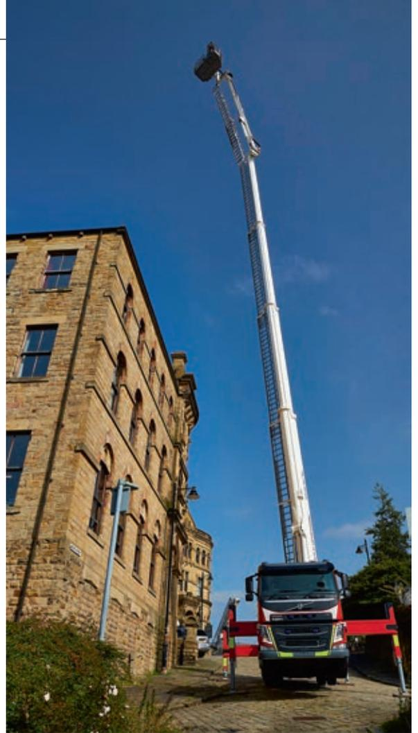
**Narrow, hilly streets are a common feature of many UK towns and cities and the F45XR has unsurpassed levelling capability with long stroke, variable jacking allowing operation on slopes up to 14 degrees**
