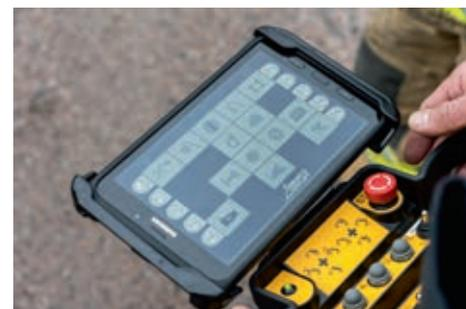
A tablet can be integrated into the remote control and serve as an additional control centre and camera display
