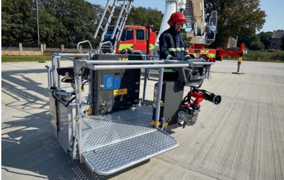
The spacious 500kg capacity cage features 60° slewing, 250kg fold down platform and can be fitted with a rescue winch and a host of other options
